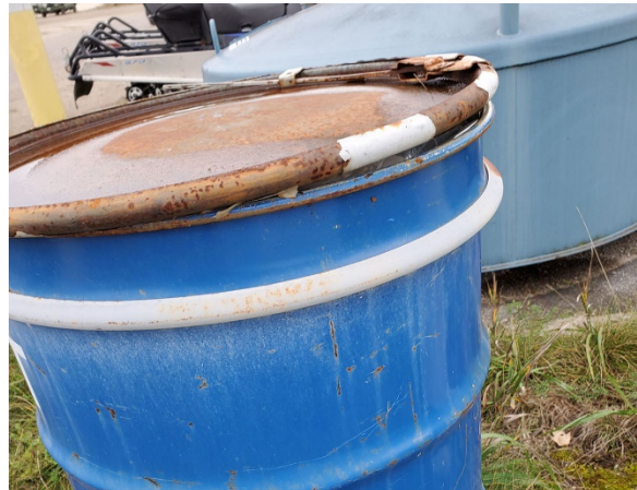
Spill kit is opened. Product appears serviceable – place into new spill drum and under cover.
